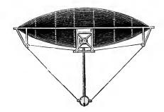
enables their position to be adjusted by means of a hand wheel. A rod which is fulcrumed below the balloon carries a hollow ball at its lower end containing sand, and by adjusting this rod forward or backward the angle of the balloon may be adjusted. By opening a valve at the lower part of the ball, sand may be discharged from same and thus serve the purpose of ballast.
